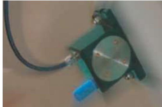
Vibration is generated by a rotor which describes an epicycloidal movement inside a steel race. OR vibrators generate a very high frequency with low consumption as compared to the force given.
